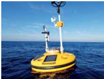
Ocean buoy and mooring for fixed-point measurements
