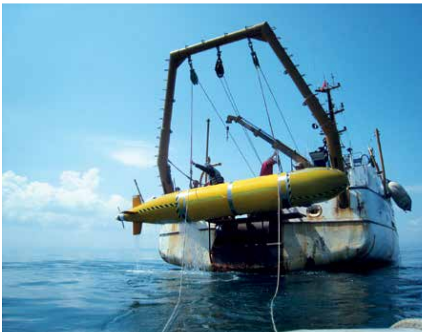
Autosub-3 being recovered from the Black Sea in 2010 onto the Turkish research vessel "Piri Reis" as part of a scientific study led by Leeds University, UK, looking at the flow in the deep saline channel from the Bosphorus to the Black Sea in May 2010
