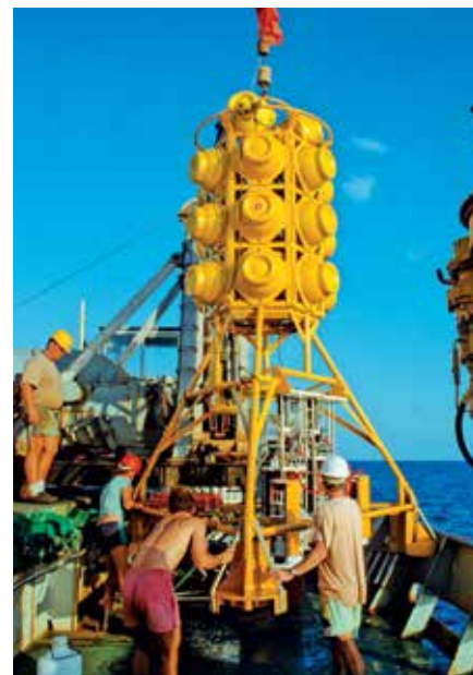
AlbeX Lander used for seafloor observation
